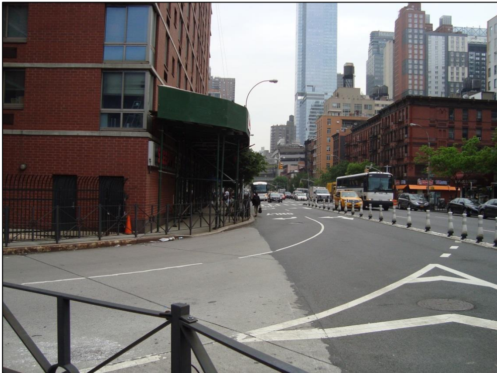
Figure 2.3.5: Fence Forces Jaywalking Pedestrian into Traffic Lanes
