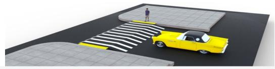
The crossing is on a wide speed bump. Its flat top is on level with the sidewalk for ADA access. A bridge at each end lets rain and snow pass below.
