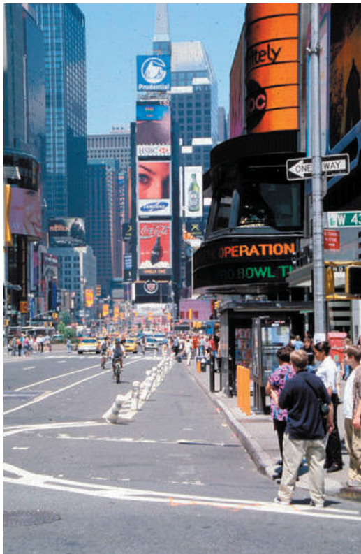
Thermal striping and plastic bollards reclaiming pedestrian space, Times Square
